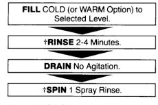
\*The RINSE SPIN Option is preset for a High Speed rinse and spin. For a Low Speed rinse and spin, touch DELICATES before selecting RINSE SPIN. This will also shorten the spin time by 2 minutes.
